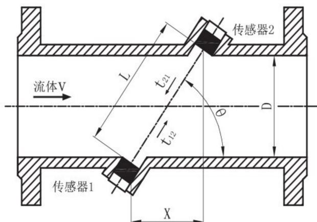
$$v = \frac{L}{2 \cos \theta} \left( \frac{1}{t_{12}} - \frac{1}{t_{21}} \right) \quad (\text{式1})$$
